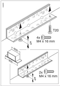
■ Fit the screws for attaching the cooker hood so that they protrude by about 5 mm, as shown.
